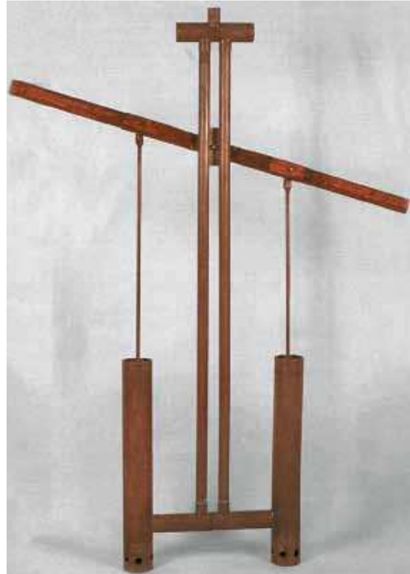
Fig. 4. Ctesibius' pump. Collection of the Society of Ancient Greek Technology. Construction D. Kriaris.
